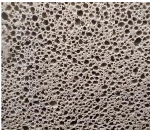
Fig. 1. Sawn cross-sections of typical RAAC structural panel.
