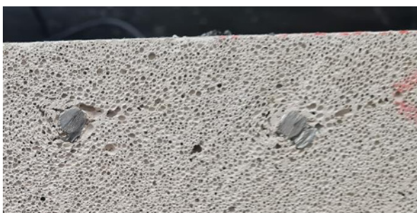
Fig. 2. Sawn cross-sections of typical RAAC structural panel, showing ‘teardrop’ shaped voids to the side of the reinforcement.
