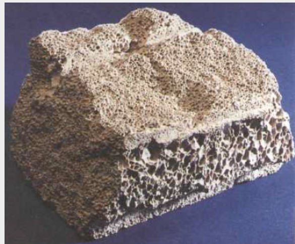
● Figure 2 A lump sample of AAC [1]
