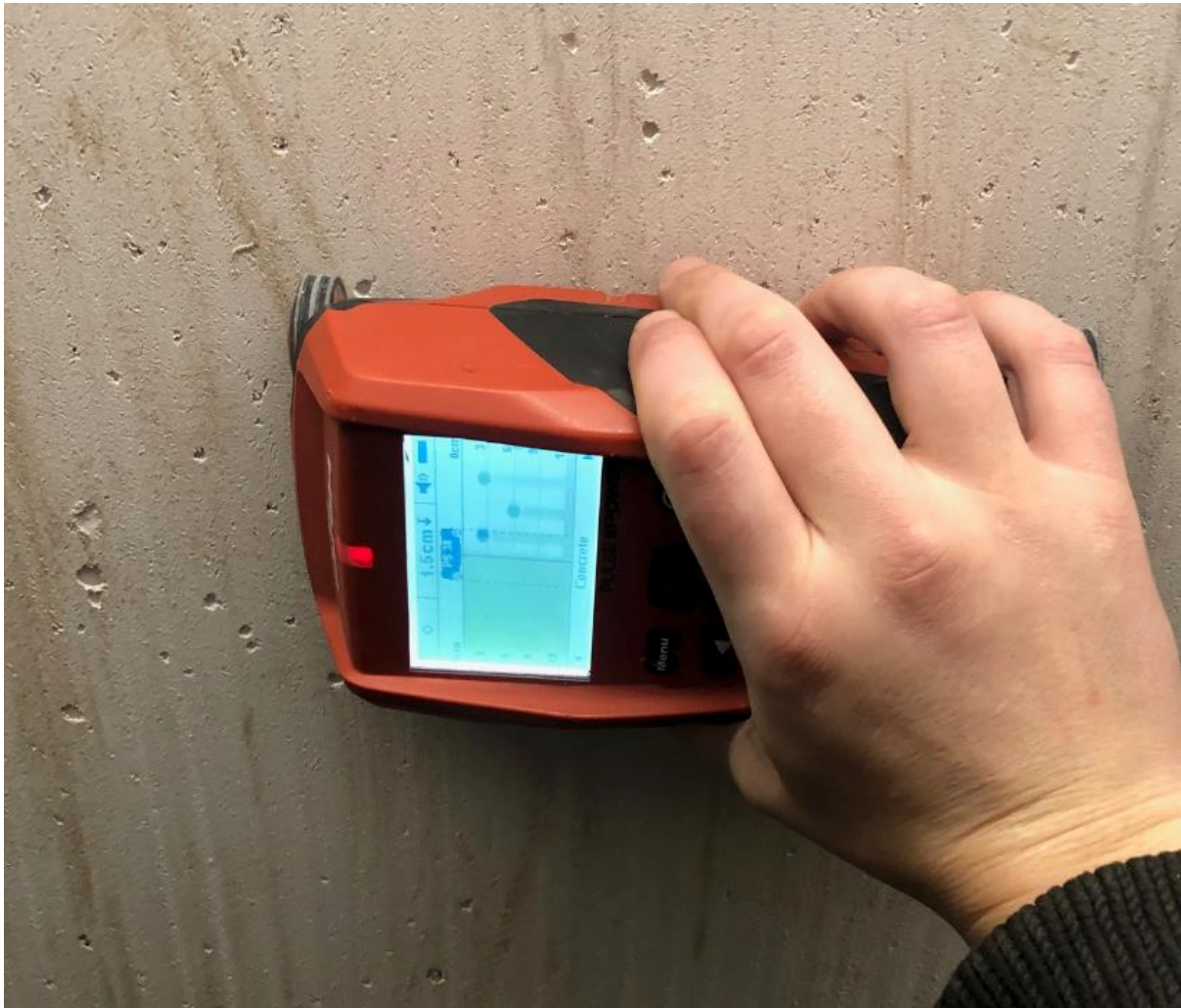
HILTI PS38 MULTIDETECTOR TAKING SITE MEASUREMENTS
